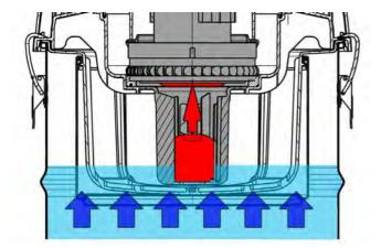
The vacuum channel is equipped with a float. If the maximum admissible wastewater level in the container is reached, the float seals against the cone of the suction turbine and the intake flow is interrupted in order to protect the suction turbine against moisture.
