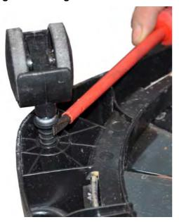
→ Pull the steering roller out of the container and replace it.
